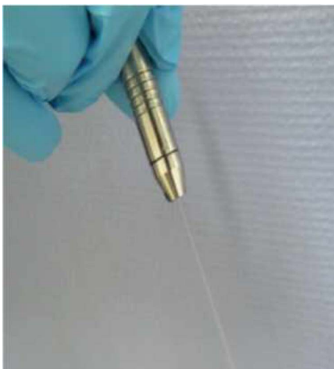
Fig. 4. Handpiece with emitted micro water jet.
