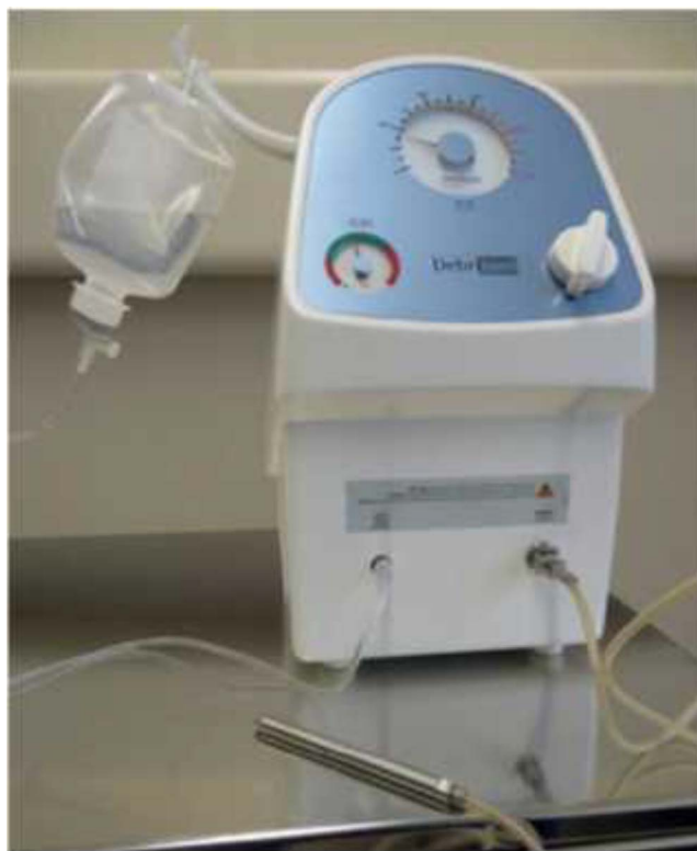
Fig. 6. MWT device. The irrigation solution is connected on the left side. The handpiece with the nozzle is lying on the table.
